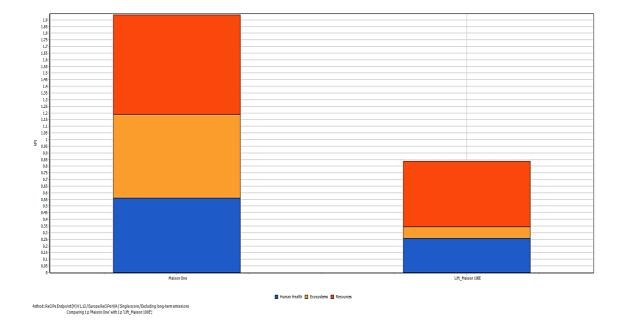
It has already been referred that the use of a lift to the total duration of life, has the greatest impact on the environment. In these charts for both models appears what shall entail this. The saving of fossil fuels, which is crucial to continuously minimize these stocks, has been significantly reduced.
