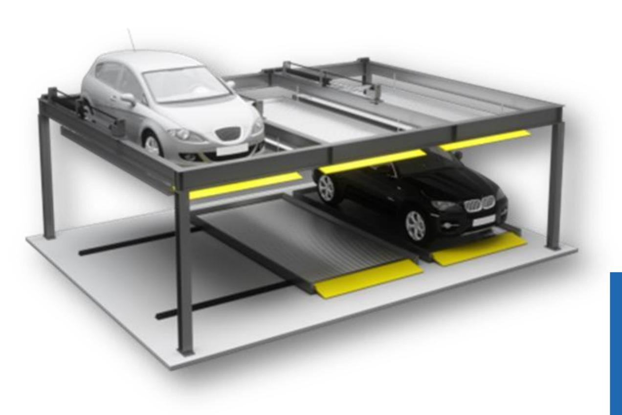
KLEEMANN **Puzzle Parking Systems** have been designed to provide a range of intelligent multi-storey parking solutions that enable independent parking of multiple cars. The selected parking space is moved to the desired position by means of an automatic control system and the parking spaces can be shifted vertically or horizontally.
